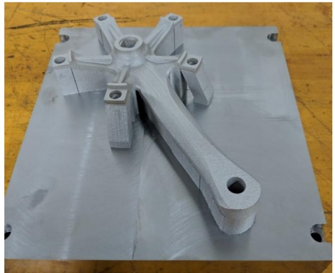
Figure 8: Parts were printed using an EOS 290, 3D metal printer
