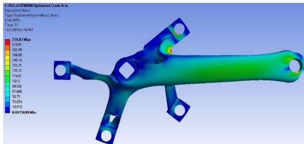
Figure 13: Stress in optimized design from FEA
