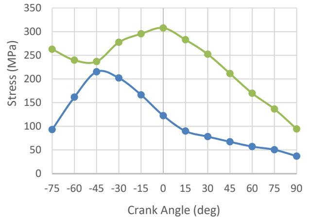
Figure 14: Comparison of maximum stress at different crank angles for the original design (blue) and the optimized design (green)
