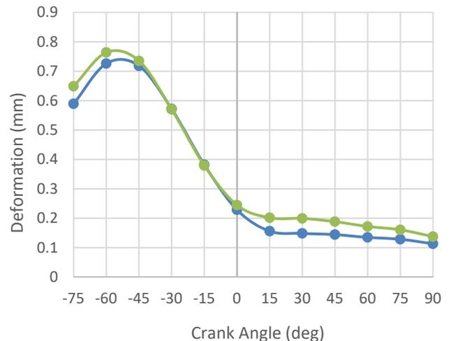
Figure 15: Comparison of deformation at different crank angles for the original design (blue) and the optimized design (green)
