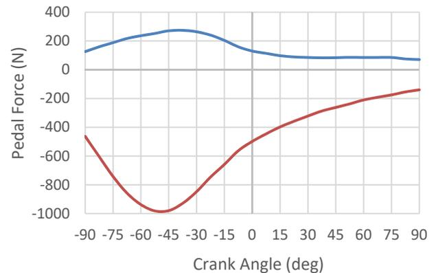
Figure 2: Pedal force toward the front of the bicycle (blue) and vertically upward (red).
