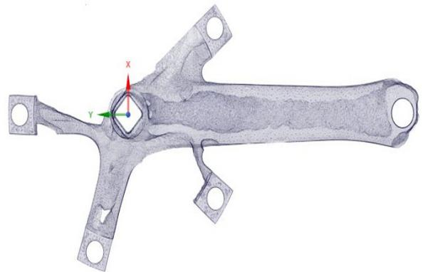
Figure 6: View of internal cavity within the optimized geometry
