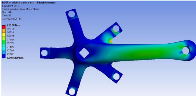
Figure 12: Stress in original design from FEA
