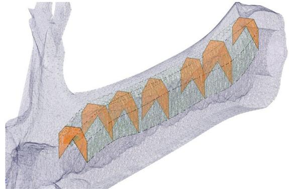
Figure 7: Design for Metal Additive Manufacturing principles were applied to make the internal cavity self-supporting
