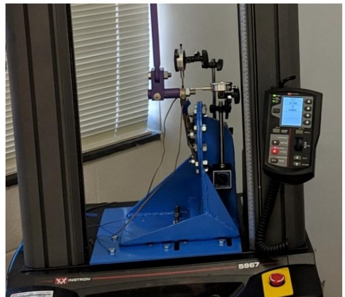
Figure 11: Each design was tested on an Instron 5967 universal testing machine at 15 degree15-degree increments
