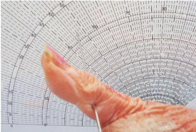
Figure 2: A K-wire through the DIP Joint (P5) was used in the experiment to measure thumb extension angle.
