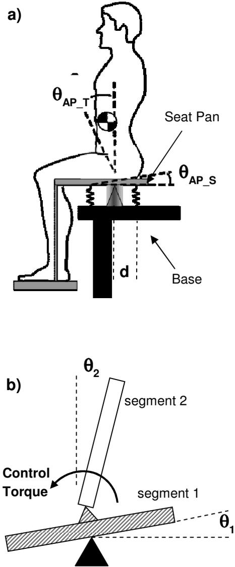
Figure 1: (a) The wobble chair is a new seated stability test apparatus where movement of the lumbar spine is used to maintain balance. (b) Two segment inverted pendulum model.
