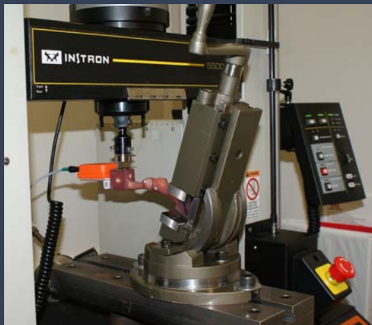
Figure 1: A custom fixture was used for cantilever testing of the first metatarsophalangeal joint fusion constructs.
