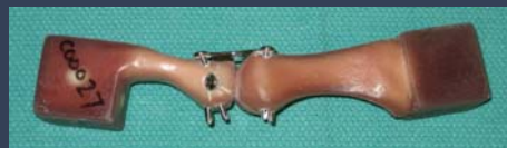
Figure 3: X-type locking plate specimen illustrating the typical mode of failure in this group: fracture through the screw tracts within the base of the proximal phalanx.
