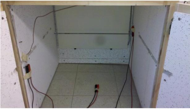
Figure 4– Thermal Enclosure with Sensors and Heater Panel
