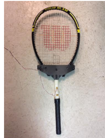
Figure 1: Instrumented tennis racket designed for the experiment.
