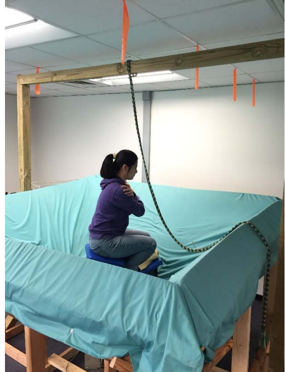
Figure 1: Experimental configuration. Participant balances on a kneeling chair in the center of a foam padded safety frame.
